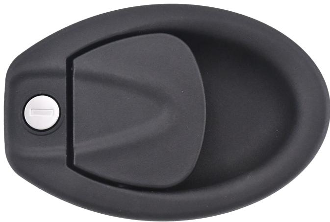
This new 030-7400 Oval Paddle Handle is designed for use on personnel and compartment doors for light to medium duty, on or off-road applications. The paddle rotation drives a plunger output which allows for a direct latch release providing a compact and low-cost access solution.
